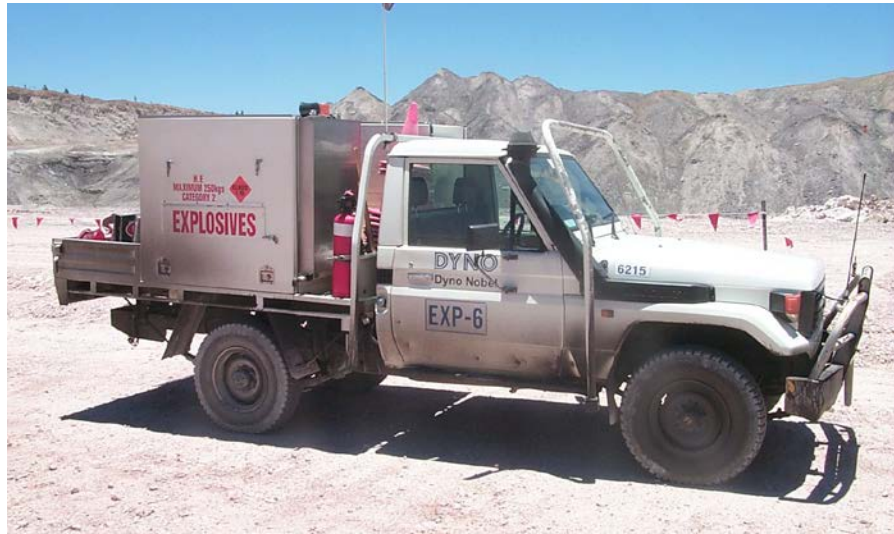
Figure 12: Explosives vehicle at a mine site with separate explosives receptacles and fire extinguishers.
