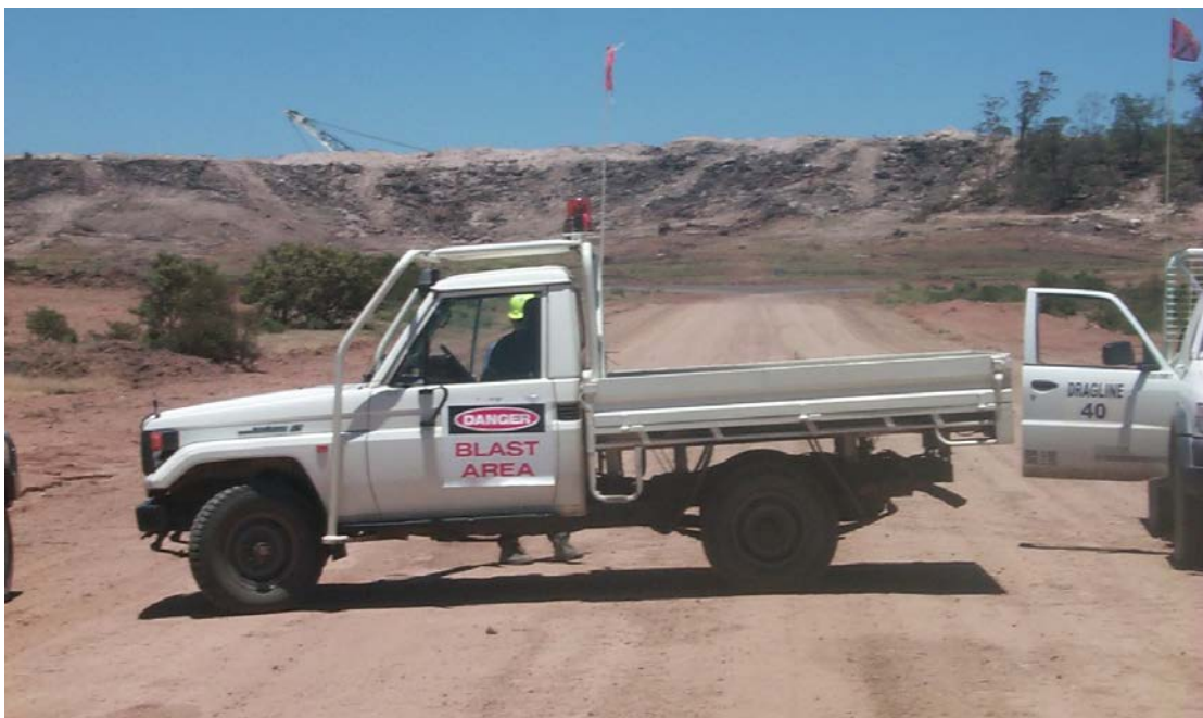
Figure 13: Access guard with signage
