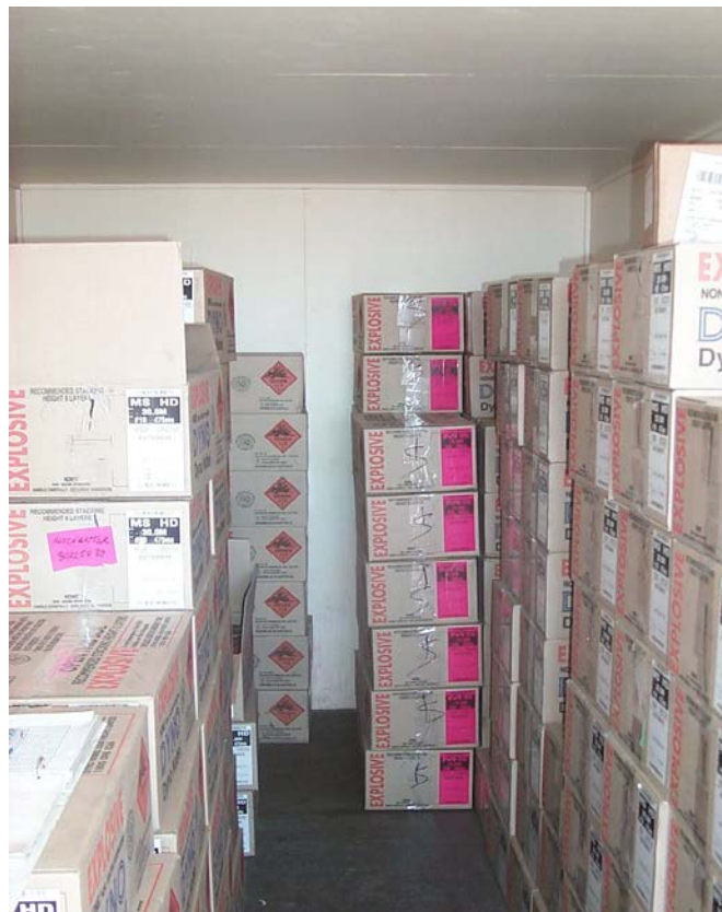
Figure 10: Explosives stacked with their labelling towards the access way for easy identification.
